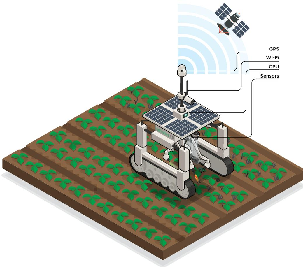
**Figure 5. Concept of an agrobot weeding mechanically with a beam of light**
