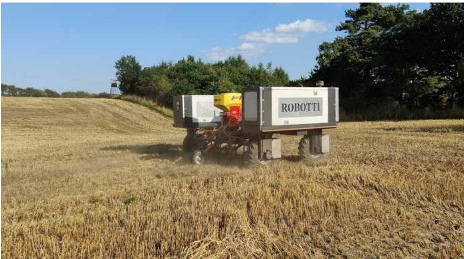
**Figure 7. Self-powered platform (Agrointelli, Denmark)**
