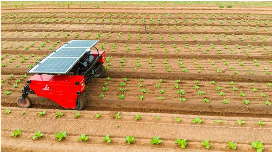
**Figure 6. Solar-powered robot (Agerris Farmhand, Australia)**
