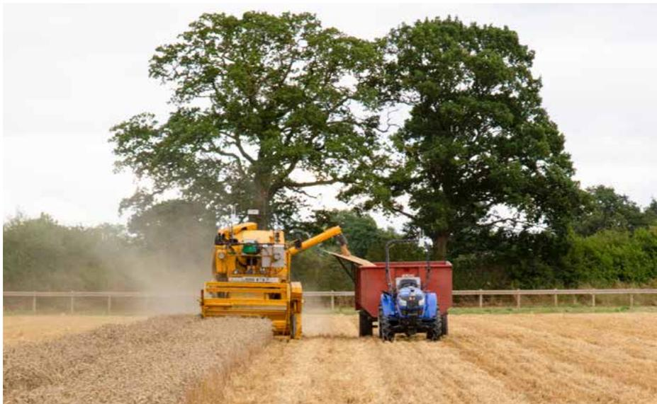
**Figure 11. Hands Free Hectare project: a 1980s harvester and a conventional small four-wheel tractor pulling a trailer**
